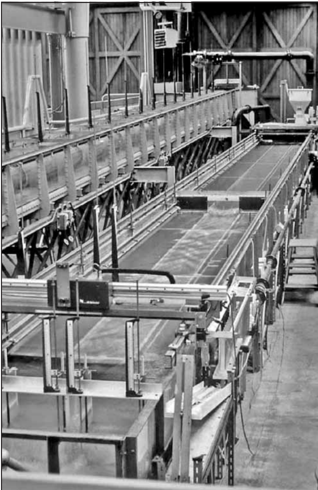
Fig. 2. Compound laboratory flume at the University of Birmingham used in testing bridge models (deck bridge model installed—from Seckin and Atabay 2005 21 )
